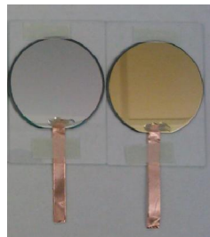
Figure 3-12. Electrowetting wafers with aluminum (left wafer) and gold (right wafer) as conductive layers.
